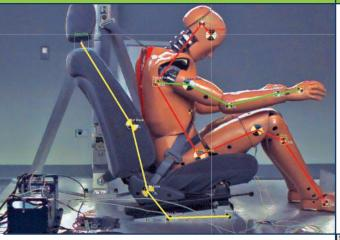
ProAnalyst enables the user to track features without having to use special markers, such as ping-pong balls, in the experimental setup. The Automatic Tracking tools find and track natural features in each video frame.
