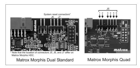
6. Connect Cable B to the J6 system reset connector of the Matrox Morphis base board (pins 3 and 4 of connector J5 for the Matrox Morphis Quad board).
