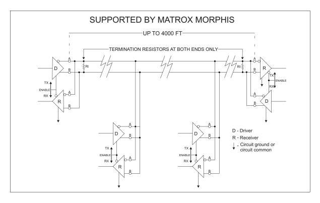
Four-wire multi-drop Matrox Morphis cannot be connected to a four-wire multi-drop network. network
