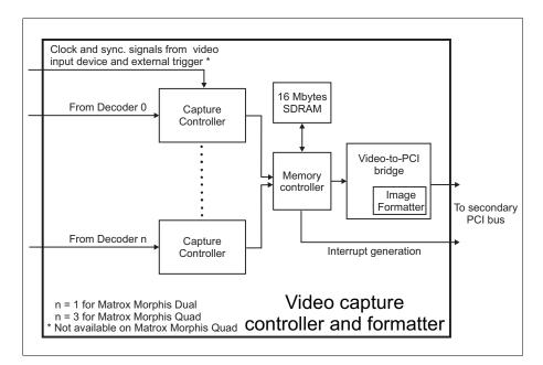
The video capture controller and formatter contains the following elements:
