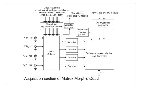
To grab from a video source, allocate a MIL digitizer with a DCF that matches the video source's data type, using the MIL-Lite function **MdigAlloc**(); a MIL digitizer represents the acquisition path(s) with which to grab from one input source of the specified type. Then, using the returned MIL digitizer identifier, call **MdigGrab**().
