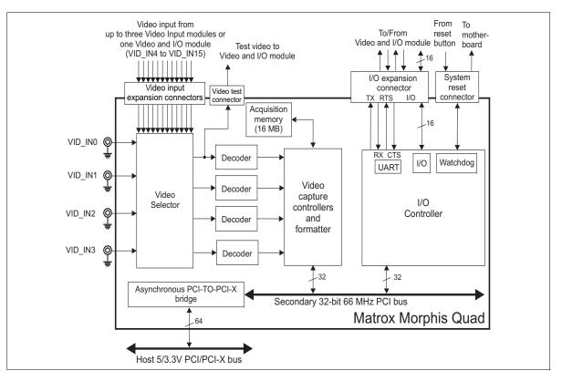
The following diagram illustrates the data flow of the Matrox Morphis Quad board.
