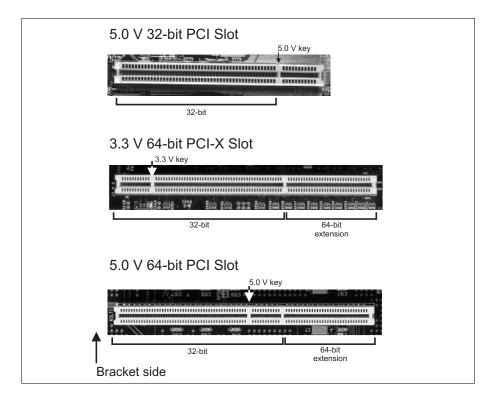
If you are also installing Matrox Morphis expansion modules, an additional slot must be available for each expansion module that you intend to install. This slot need not be adjacent to the base board. In addition, the slot can be of any type because the expansion modules' support tab(s) can be removed; if a PCI/PCI-X slot is selected, the tab(s) will fit into the slot's connector, ensuring that the module does not move.
