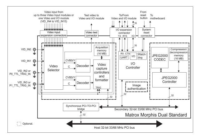
The following diagram illustrates the data flow of the Matrox Morphis Dual HDC board.
