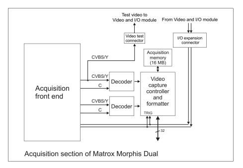
The following diagram illustrates the main components of the acquisition section of Matrox Morphis Dual.
