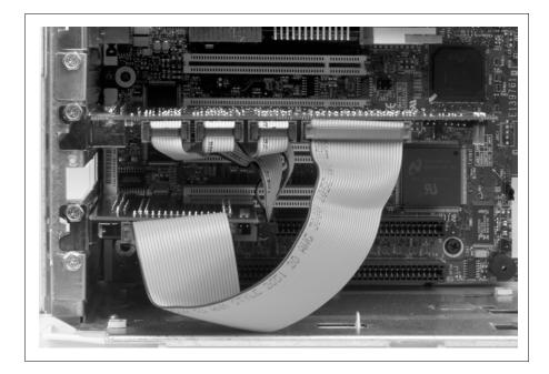
7. If you expect to test the video inputs arriving on the base board, connect the video test connector of the module to the video test connector of the base board using a custom cable. This connection allows you to output any of the CVBS video inputs, or the Y component of any Y/C video inputs, arriving on the base board (those from the Video and I/O module or those directly from the base board).
