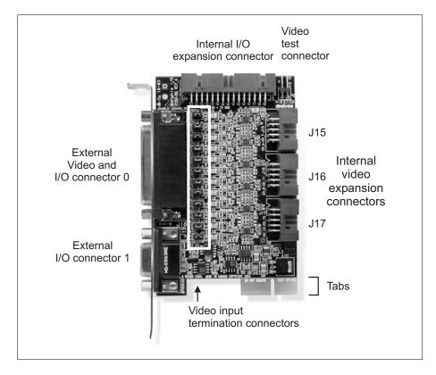
To break off the tabs, use a set of pliers; there is a groove along the tabs so that you can break them off without an excessive amount of force.
