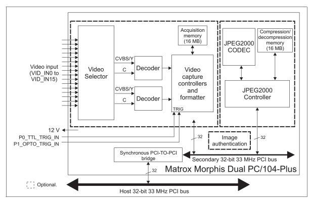
The following diagram illustrates the data flow of the Matrox Morphis PC/104-Plus board.
