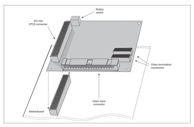
3. Carefully position Matrox Morphis Dual PC/104-Plus over the connectors and press the board firmly into place.
