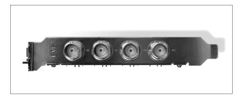
You can use a standard BNC to BNC video cable (available from your local electronic store) to interface a composite color or monochrome video source with one of these connectors. To interface a Y/C video source, you can use a custom cable, or you can use two BNC to BNC cables and a Matrox BNC-TO-SVHS adapter cable.
