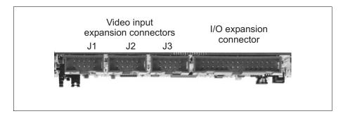
7. Repeat steps 2 through 6 for each Matrox Morphis Video Input module that you need to install. You can install up to 3 Matrox Morphis Video Input modules.
