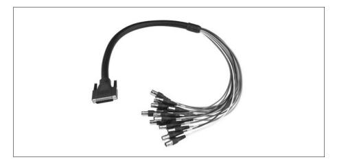
• An HD-44M-18BNC+ input cable, a 3-foot cable with a 44-pin male connector at one end and eighteen BNC female type connectors at the other end. This cable is used with Matrox Morphis Dual PC/104-Plus
