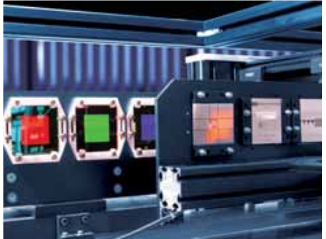
The A300f is measured by the CTT+ according to the EMVA 1288 standard
