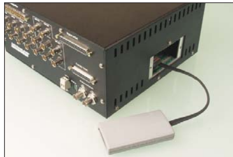
Figure 13. Removable side panel allows direct access to the JTAG port for program development and debug purposes. LEDs are also viewable for debugging through this panel.
