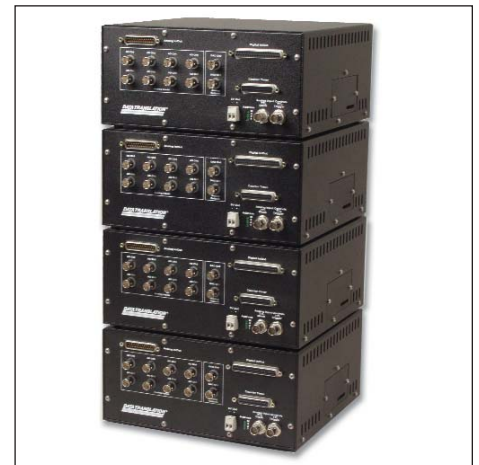
Figure 11. Up to 4 Sleek Boxes can be configured for high channel count systems.
