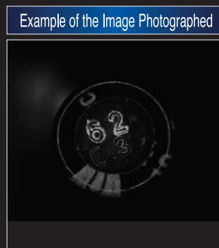
Dirt on the shrink as well as characters on the top plane of a capacitor can be recognized simultaneously. Work: Electrolytic capacitor Light: IDR-T75/46B-1
