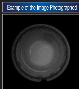
Defects on a product can be detected by irradiating uniform light from above. Work: Cap of a PET bottle Light: IDR-90/50DW
