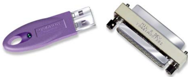
Figure 1: Hardware key (dongle) for USB (left) or the parallel port (right).
